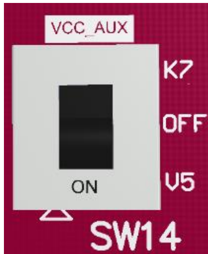
Figure 15 – VCC_AUX Voltage SW14
