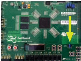
Figure 3: Setting FMC IO Voltage to 2.5 V
