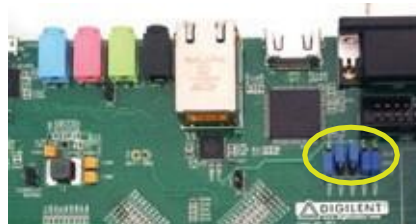
Figure 4: Setting boot-mode jumpers to boot from the SD card
